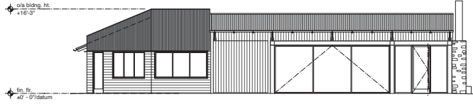
Roof, Gutters & Downspouts Corrugated metal roof half-round metal gutters, gutter straps every other rail; mt-factory-applied Charcoal Gray Color
