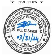
THE ENGINEERING SEAL COVERS STRUCTURAL DESIGN ELEMENTS PRESENTED IN THIS SET OF PLANS. IT DOES NOT PROVIDE ANY ARCHITECTURAL, SITE, ZONING, HVAC, ELEC, MECH DESIGN OR REQUIREMENTS. THESE ITEMS MUST BE ADDRESSED BY THEIR RESPECTIVE PROFESSIONALS IN CHARGE.
